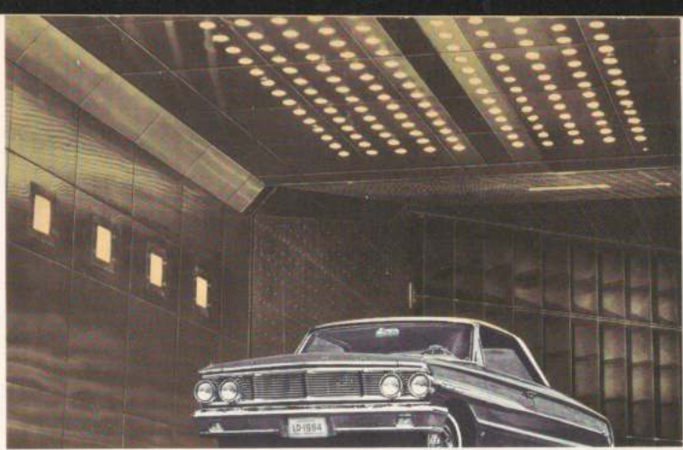
To test "sun load" conditions, 240 overhead lamps can pour blistering heat on every exposed square foot of the test car.
